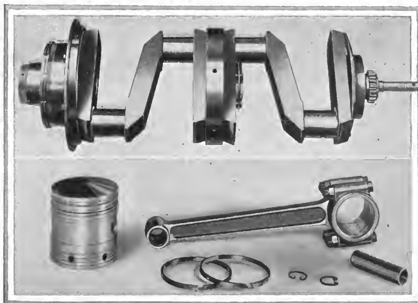
Above—Two-piece crankshaft used in the new Premier racers. It is carried on four ball bearings, the rear bearing being double Below—Piston and connecting-rod assembly of the new Premier racers. Although 2 lb. lighter than the Peugeot assembly, it is stated to be stronger
